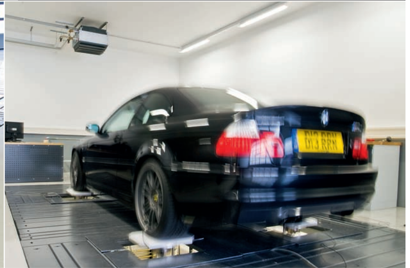
KW's 7-post rig allows accurate race track replications as well as suspension optimisation testing. Here, KW tests an M3 CSL after fitting a custom kit made up of clubsport and race components
