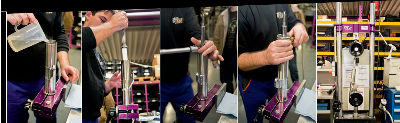
The damper cylinder is partially filled with oil before the rod is inserted. Once the unit's assembled, oil is pumped in under pressure to fill the completed damper before being tested on a shock dyno
