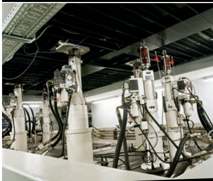
KW's 7-post rig allows accurate race track replications as well as suspension optimisation testing. Here, KW tests an M3 CSL after fitting a custom kit made up of clubsport and race components
